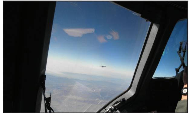
The first C-17 flight tests employing vortex surfing were conducted at Edwards Air Force Base, Calif., Sept. 6 and Oct. 2. Surfing Aircraft Vortices for Energy, or \$AVE, involves two or more aircraft flying together for a reduced drag effect to save fuel. (Courtesy photo)
