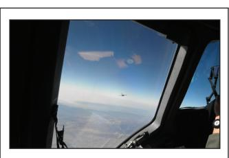
The first C-17 flight tests employing vortex surfing were conducted at Edwards Air Force Base, Calif., Sept. 6 and Oct. 2. Surfing Aircraft Vortices for Energy, or \$AVE, involves two or more aircraft flying together for a reduced drag effect to save fuel. (Courtesy photo)
